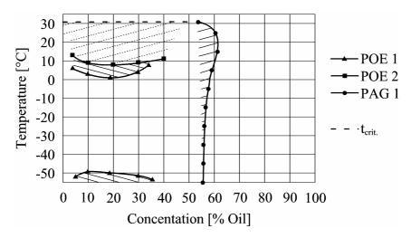
**Figure 8** Miscibility limits CO<sub>2</sub> / POE & PAG at sub-critical temperature conditions (DEA development products)
