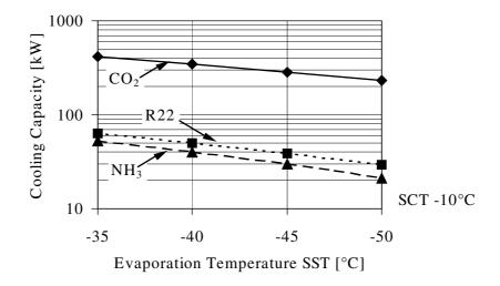
Figure 9 Performance behaviour of a screw compressor with 220 m<sup>3</sup>/h displacement
