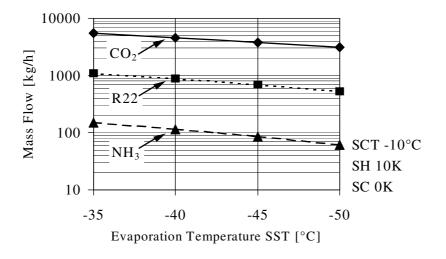
Figure 11 Comparison of mass flow (screw compressor with 220 m<sup>3</sup>/h displacement)
