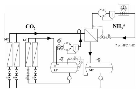
Figure 1 Cascade system with CO<sub>2</sub> (simplified sketch)
