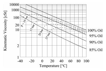
**Figure 7** CO<sub>2</sub> solubility in POE oil and the resulting kinematic viscosity (DEA development product)
