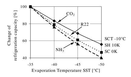
Figure 10 Relative change of Refrigeration Capacity with regard to SST - 35°C and SCT -10°C
