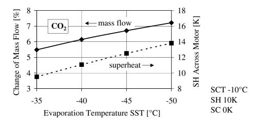
Figure 6 Suction superheat across the motor and the resulting change in mass flow
